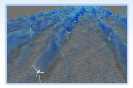
Detailed computer simulations such as this one using SDSC's Trestles system allow researchers to study the flow in wind-farms in great detail. This image shows a visualization of the flow in a very large wind-farm. The blue regions indicate the low velocity wind-speed regions (wakes) formed behind the turbines. *Visualization by David Bock (NCSA)* as part of XSEDE's Extended Collaborative Support Services.
