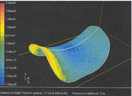
High Speed Conveying Create Vortices Shedding... ...'Rocking Chips' NOT GOOD!
