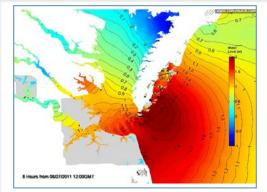
A snapshot of an animation for water level prediction including the wind-wave signature.
