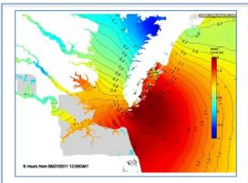
A snapshot of an animation for water level prediction including the wind-wave signature.
